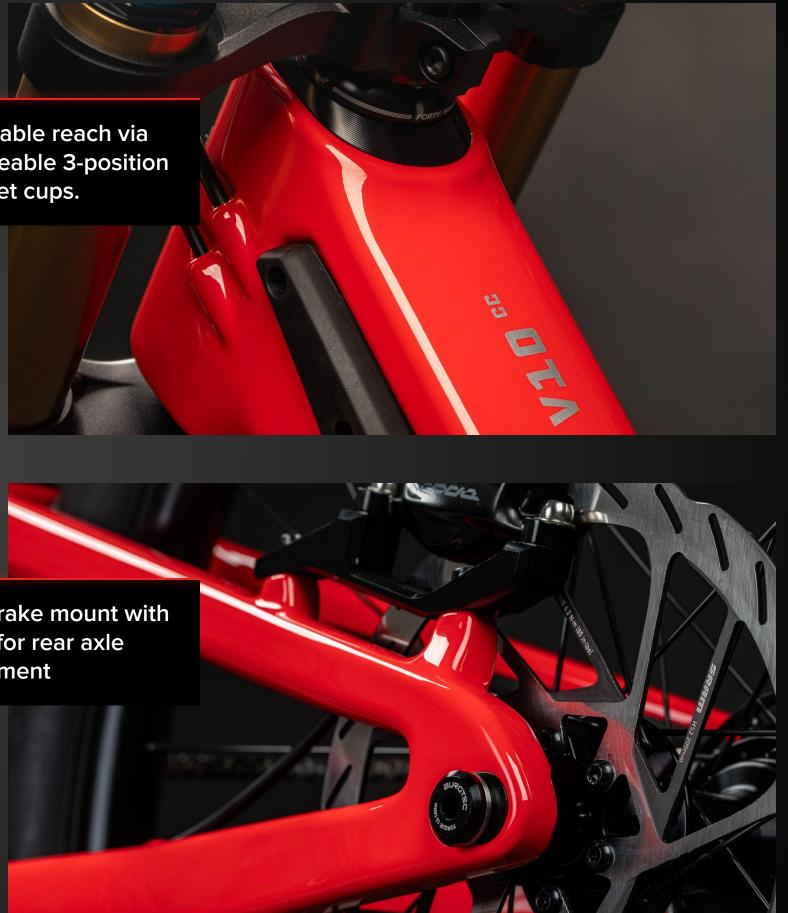
slider for rear axle adjustment
