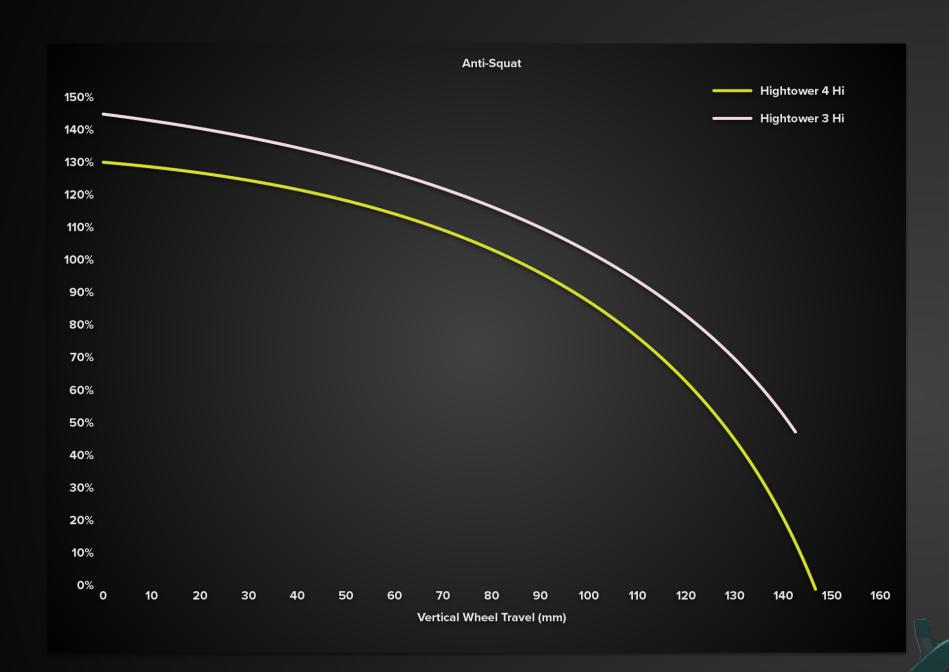
Anti-squat refers to how much your pedaling inputs stiffen the suspension. Too little and you have a bike that bobs under power. Too much and the bike will be harsh and not as able to absorb bumps while under power
